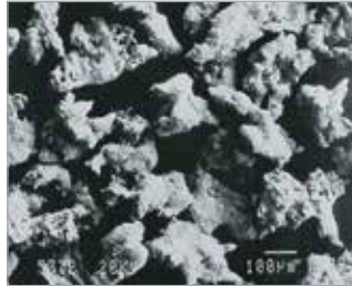
AMETEK P316L stainless steel filter powder screened to precise mesh sizes for optimum spinning quality and throughput.
